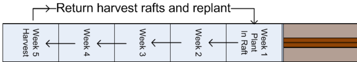
Figure 17 - Weekly rotation of rafts in deep water culture
